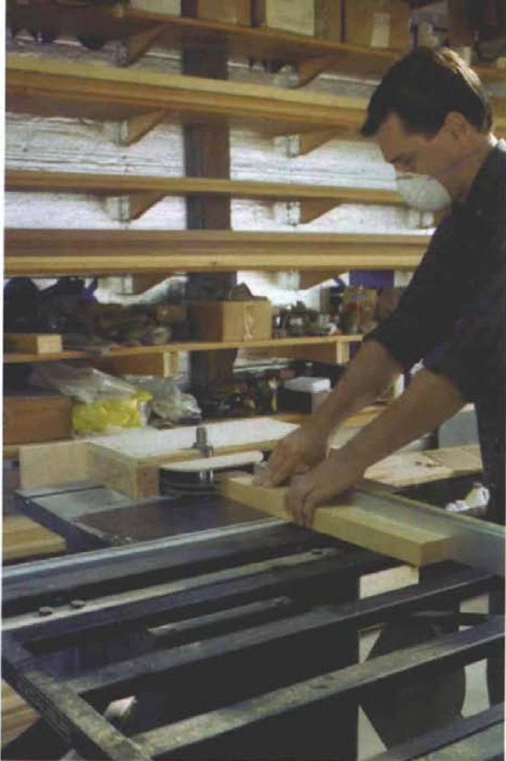
Tenon cheeks were cut on a shaper. Both cheeks of the tenon were cut simultaneously with sawblades mounted on the shaper spindle. The shaper's speed was geared down for this operation.
