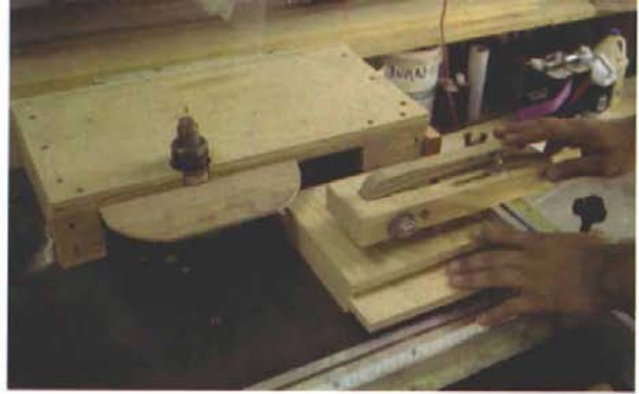
A cam clamp mounted on the sliding fence holds short pieces safely while tenoning. Some parts, such as the top and bottom rails of sidelights, were too small to hold by hand. Downward pressure on the cam lever clamps the workpiece to the shaper's sliding table.
