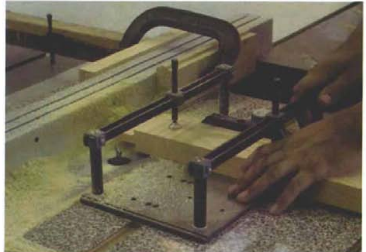
Rails were coped on a router table with a sliding carriage. The ends of the rails were coped with a profile opposite that of the stiles. Note the stop block clamped to the table for registration.
